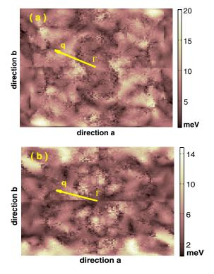
FIG. 2 (color online). Calculated phonon-momentum dependence of the moduli of the *e*-ph vertex functions in the a - b plane for (a) electrons at the bottom of the LUMO band, and (b) holes at the top of the HOMO band, interacting with phonons of the lowest optical branch (the zone-center energy is 11.4 meV).
