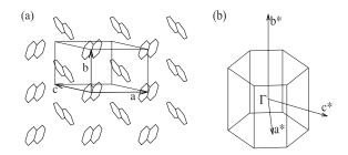
FIG. 1. (a) An illustration of the crystal structure of naphthalene, comprising molecular layers (in the a - b plane) stacked in the crystallographic *c* direction. Each unit cell contains two inequivalent naphthalene molecules in a herringbone-like arrangement. (b) The irreducible wedge of the Brillouin zone in the naphthalene crystal. The zone center ( $\Gamma$ -point) is indicated, along with the reciprocal basis vectors.
